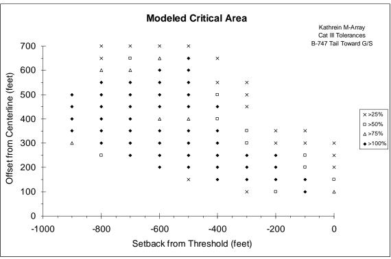
The chart just above shows the Kathrein Antenna with a 747 parallel to the runway with the tail towards the tower (CAT III tolerances). M-Array tower at 400 feet offset.
