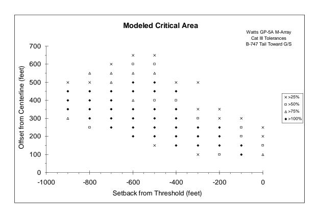
In the chart just above we have the Watts GP-5A with a 747 parallel to the runway with the tail towards the tower (CAT III tolerances). M-Array tower at 400 feet offset.
