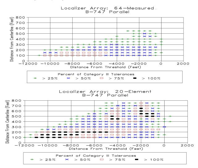
The aircraft was modeled parallel to the runway and perpendicular to the centerline in 435 positions in each orientation for a total of 870 cases. Modeling results confirmed a substantial reduction of the ILS critical area, suggesting considerably greater airport development opportunities when a wide aperture ILS is employed.
