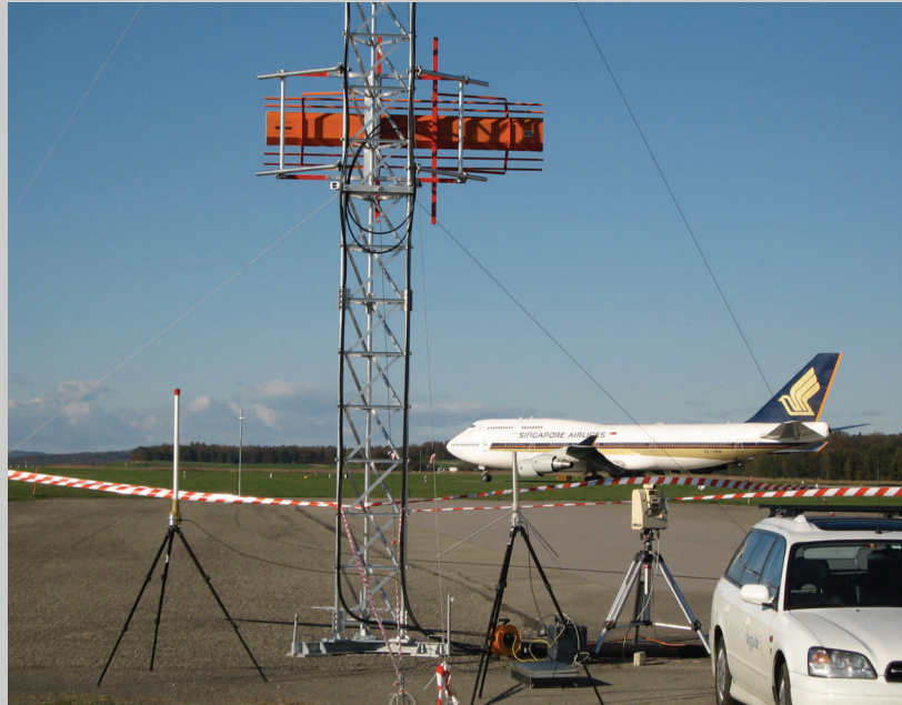
Critical Area Tests Conducted in Zurich Switzerland with a 747 Aircraft Watts GP-5A Image Glide Slope Antenna Element in an M-Array
