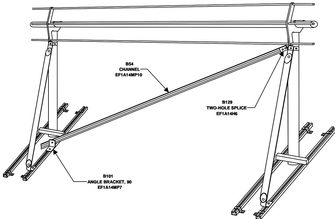
Figure 9-10. Antenna Support, Rear View (Including Transverse Brace)
