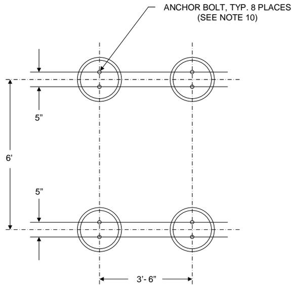
Figure 9-5. Monitor Pilings, Detail "D"
