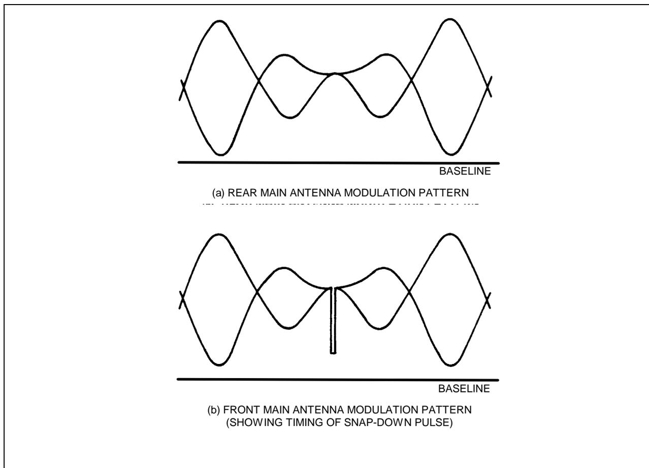
**Figure 9-30. Front and Rear Main Antenna Modulation Patterns**
