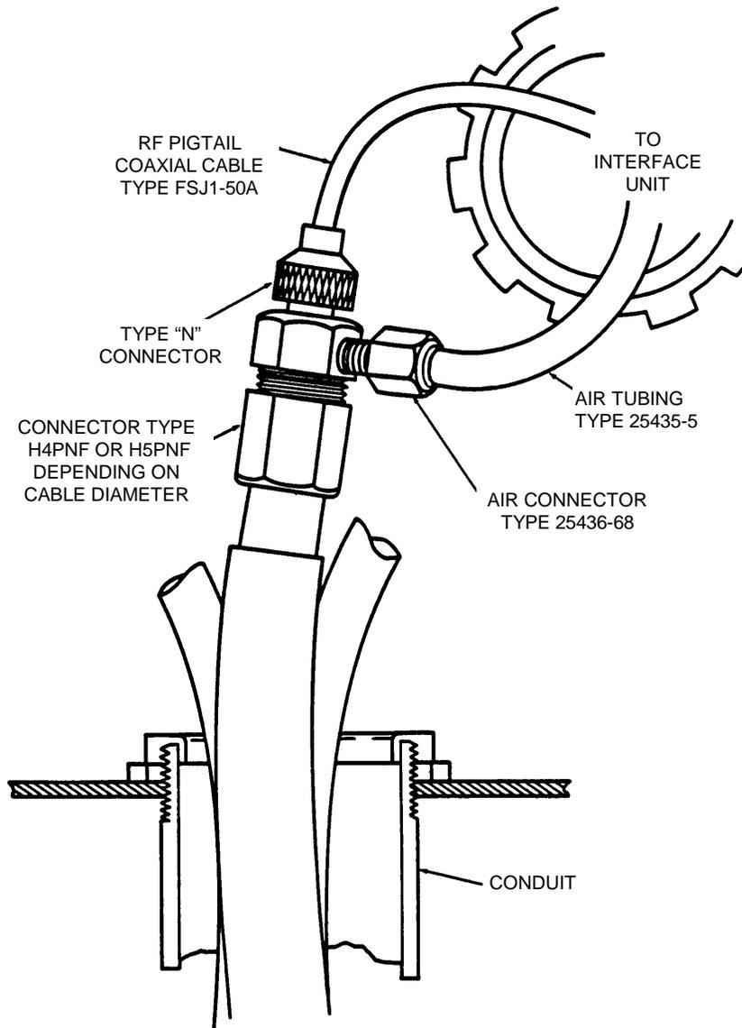
Figure 9-25. Typical Cable Termination in Outside Junction Box
