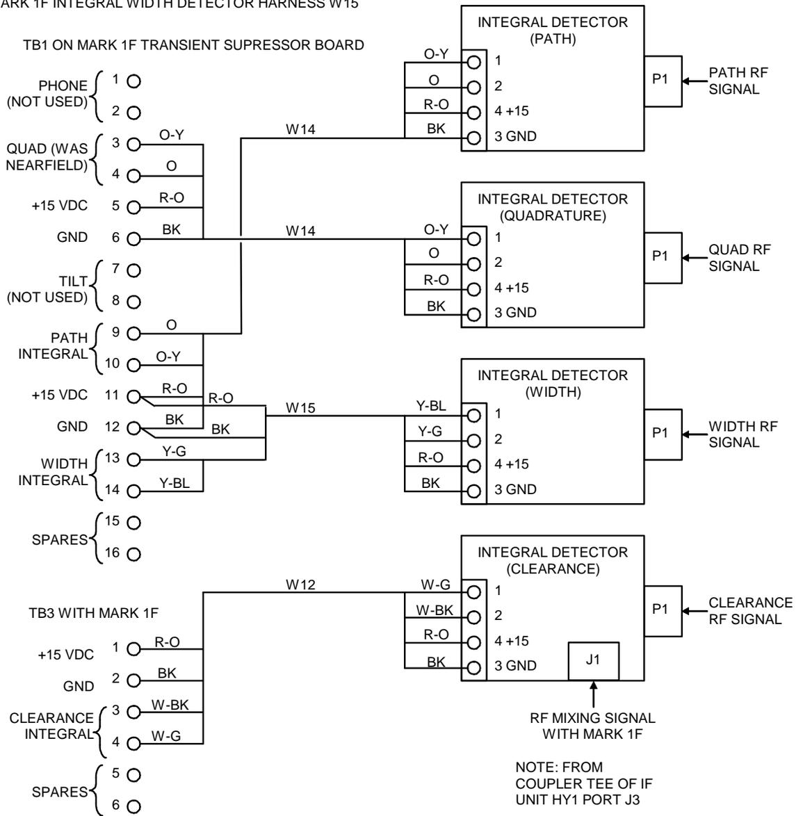
NOTE: IF THE MARK 1F TRANSIENT SUPPRESSOR BOARD IS NOT USED, DETECTOR CONNECTIONS CAN BE MADE ON THE IF UNIT TBI.
