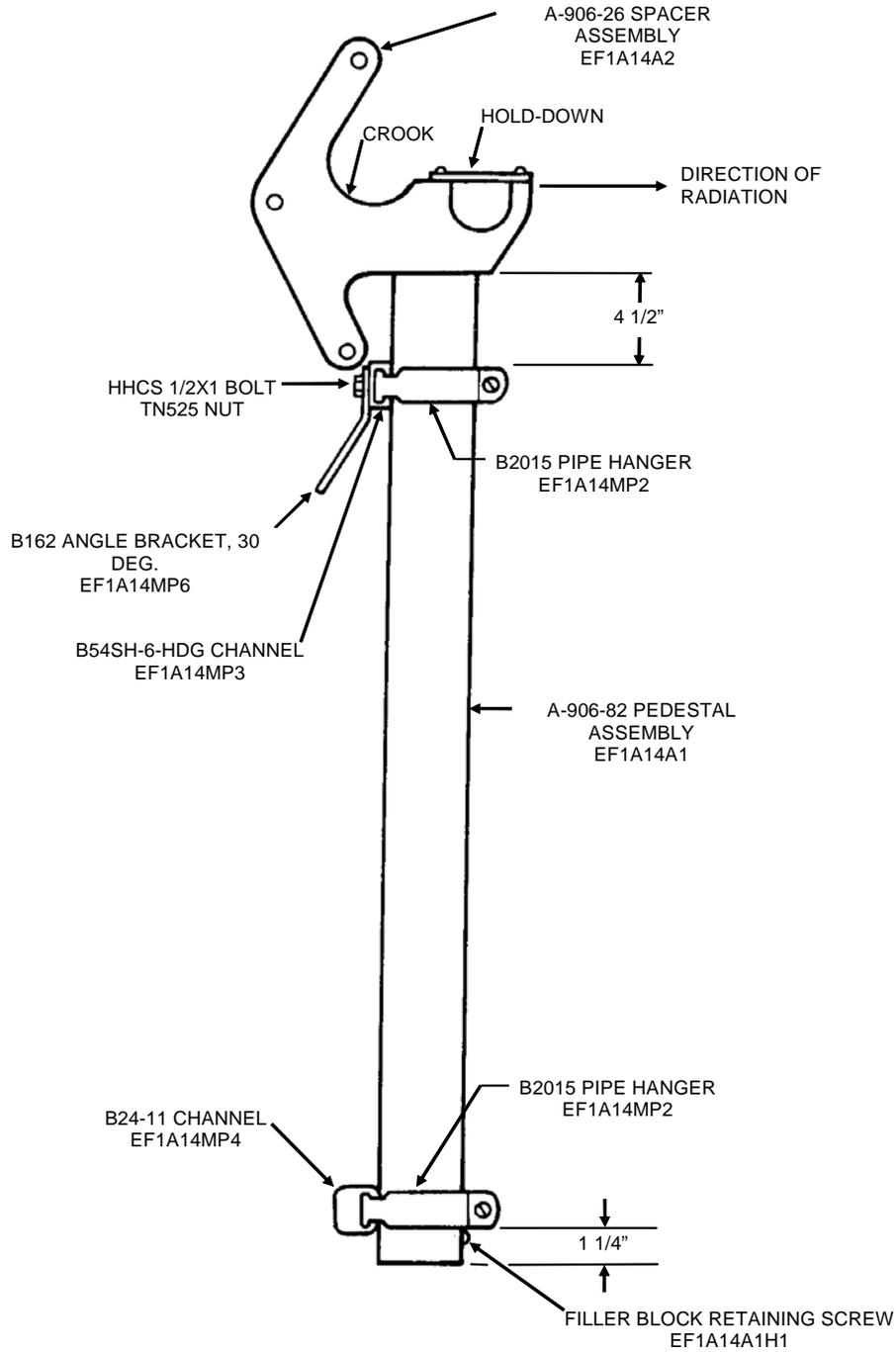
Figure 9-7. Pedestal/Spacer Assembly
