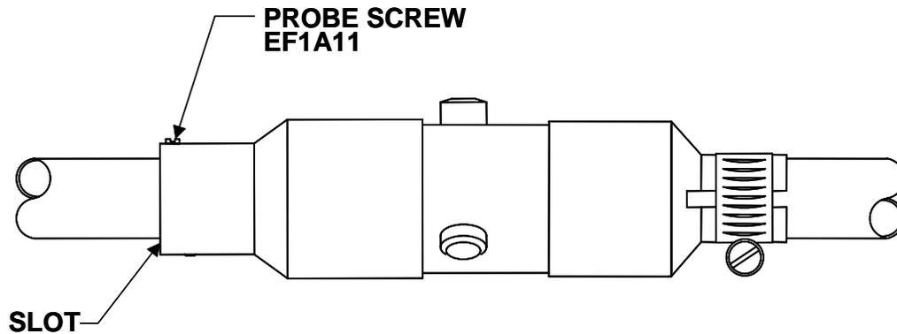
Figure 9-12. Radiating Structure Showing Probe Screw and Slot (Radome Removed)
