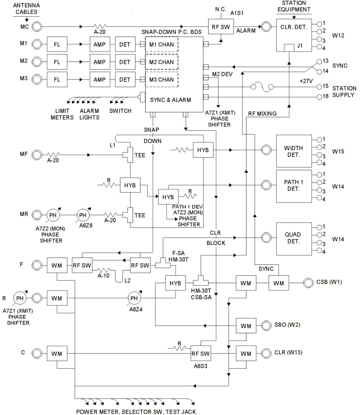
Figure 9-28. Interface Unit, Partial Block Schematic
