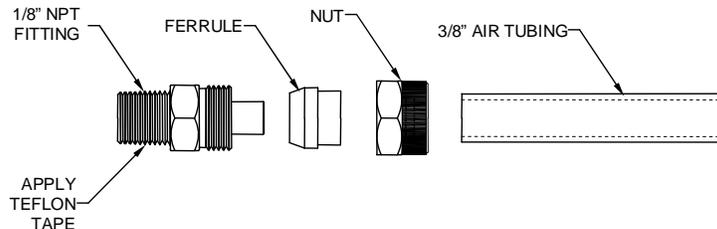
**Figure 9-26. Air Connector Type 25436-68 Installation**
