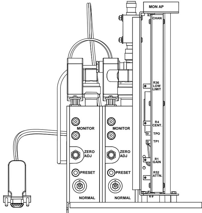
Figure 9-33. Autophaser Assembly, Type AP-105, Front View
