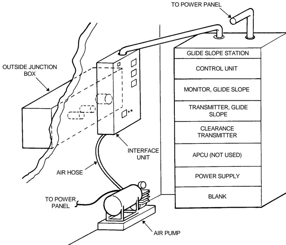
**Figure 9-19. General View of Typical Station Equipment**
