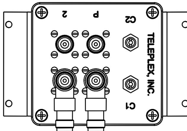
**Figure 9-31. Teleplex Hybrid, Main Bridge (shown as mounted in interface unit)**
