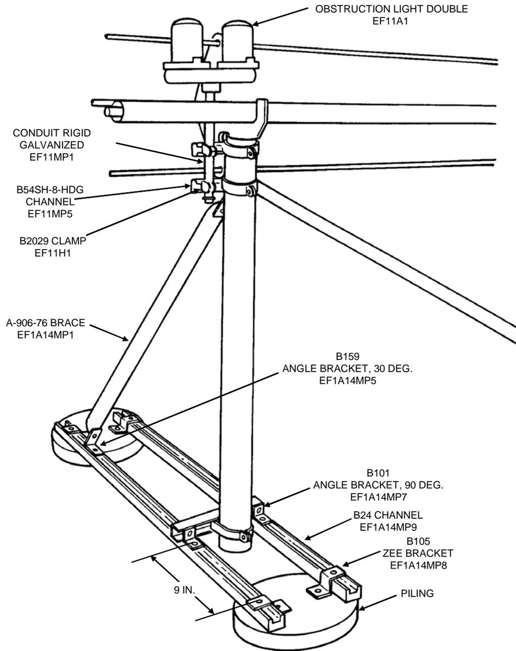
Figure 9-8. Antenna Support, Front View (Including Obstruction Light)
