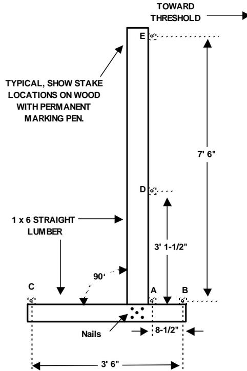
Figure 9-4. Pedestal Layout Template, Detail "C"
