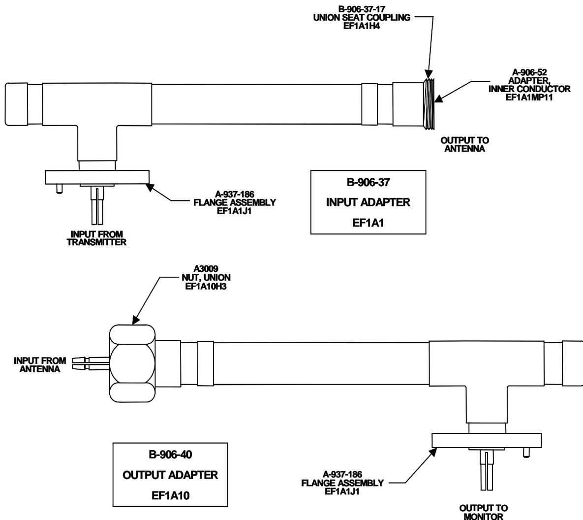
**Figure 9-14. Front and Rear Main Antenna, and Clearance Antenna Input and Output Adapters**
