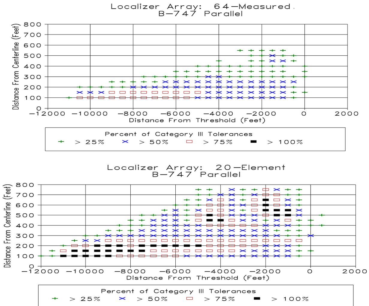
The aircraft was modeled parallel to the runway and perpendicular to the centerline in 435 positions in each orientation for a total of 870 cases. Modeling results confirmed a substantial reduction of the ILS critical area, suggesting considerably greater airport development opportunities when a wide aperture ILS is employed.
